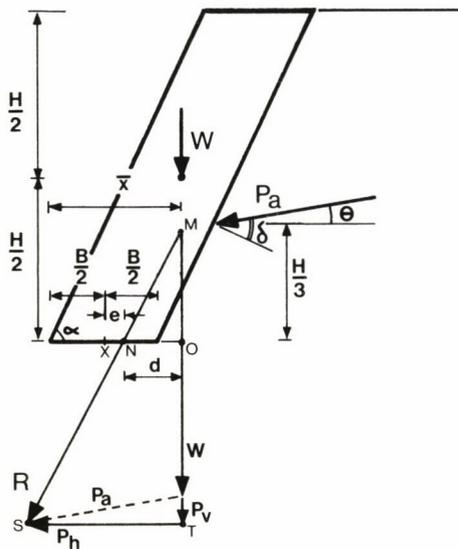
Fig. 3. Idealised section of upper  $H$  metres of wall
