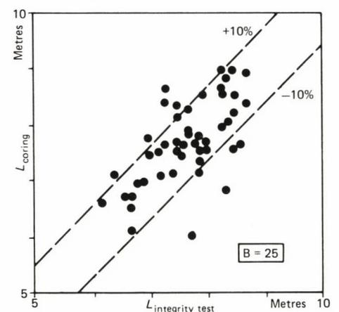
Fig. 5. Comparison of pile length
