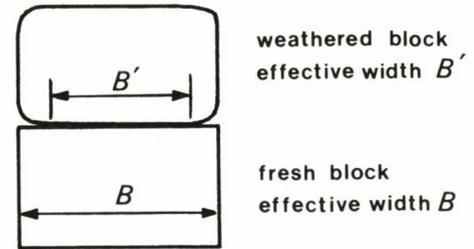
Fig. 4. Effect of weathering on block width
