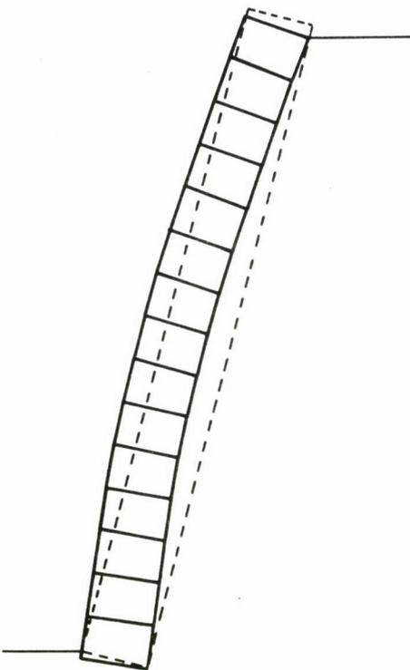
Fig. 7. Bulging failure on a compressible base
