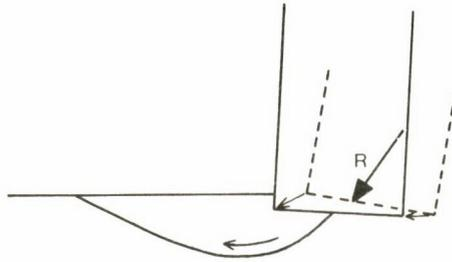
Fig. 8. Displacement of wall base due to bearing capacity failure
