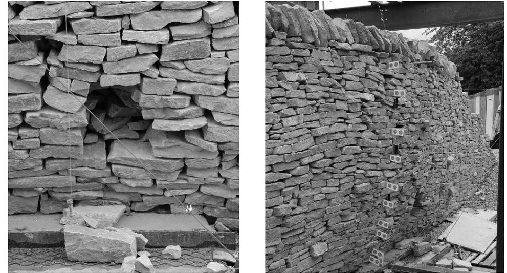
Figure 6: Test wall 3: a) local failure; b) prior to total failure
