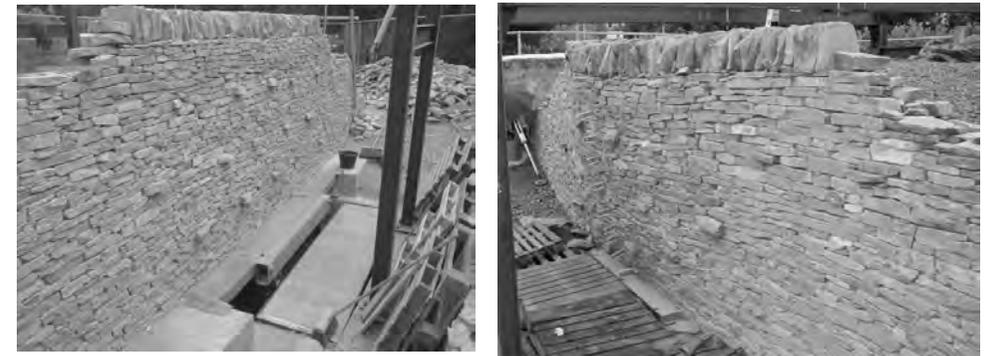
**Figure 3: Test wall 1: a) post construction; b) prior to failure**
